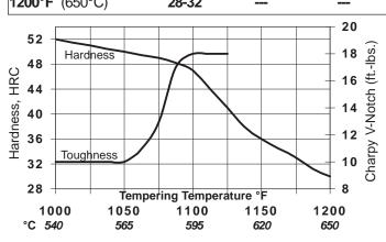
(\*) Longitudinal Toughness Measurements
